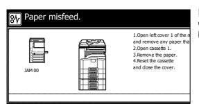
If a paper jam occurs, the touch panel will display *Paper misfeed* and the copying will stop. Refer to these procedures to remove the jammed paper.
